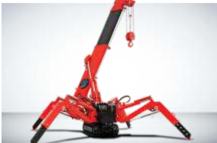
Mini Crawler Crane Capacity: 2T - 7T
