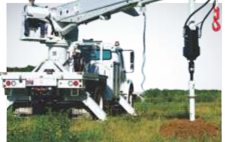
Digger Derrick Sheave Height 32m, Lifting Capacity: 27.2
